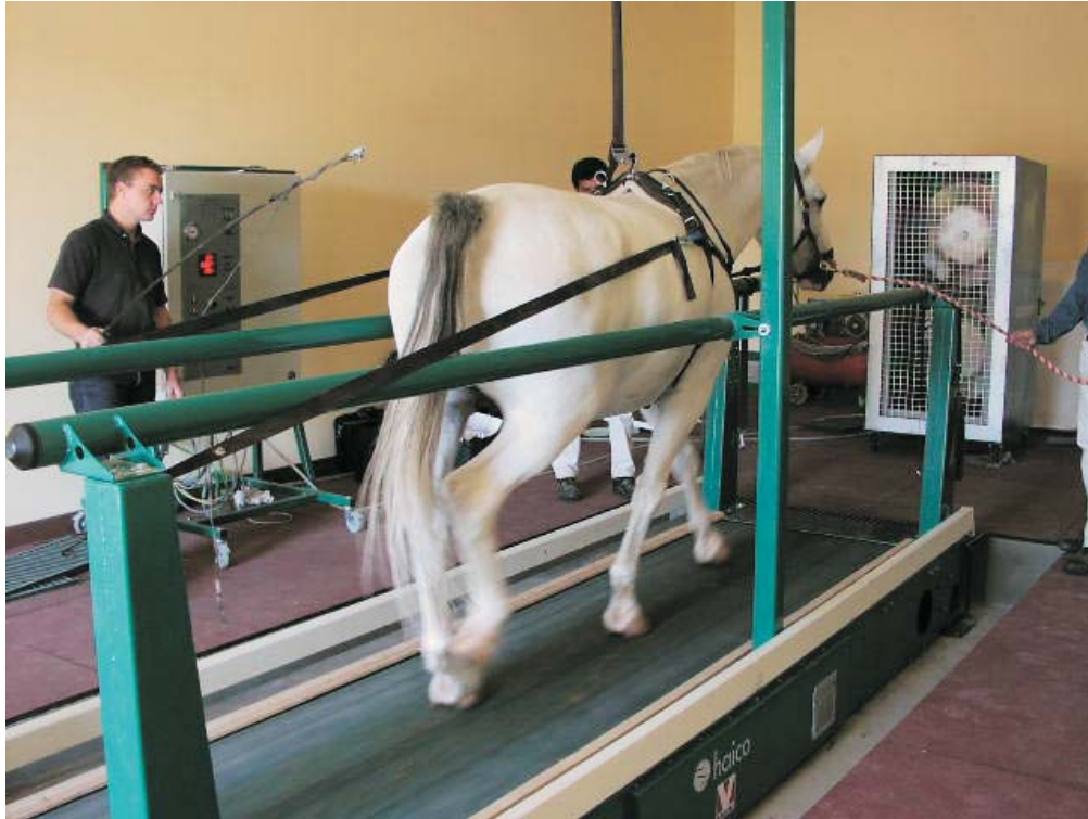
Inside built automatic pulling load unit system
