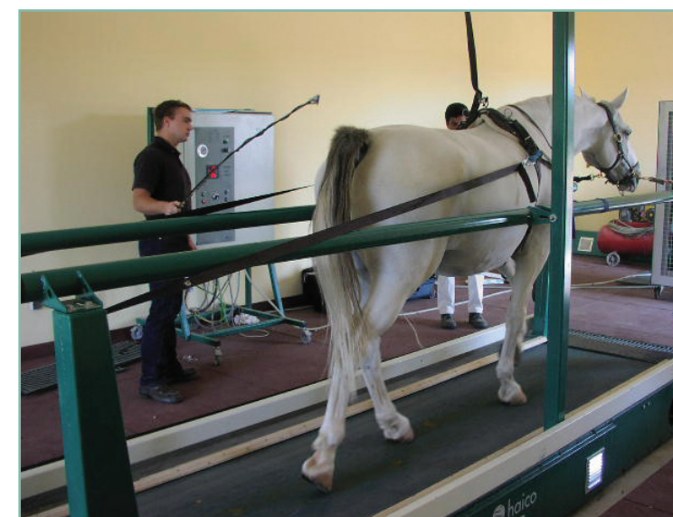
Pulling belts are connected to the safety harness and the pulling force can be steplesly adjusted between 0 to 85 kg (850N) manually or automatically via the test programs.
