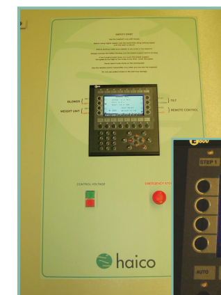
Clear and logical control unit. Standard / individual test program enables comparable test results between horses.
